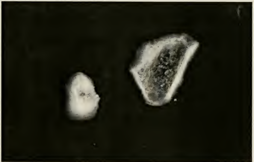
Figure 4.17 Reference sample of quartz. Note resemblance to sample 1.04-1 above. Magnification 100X.
